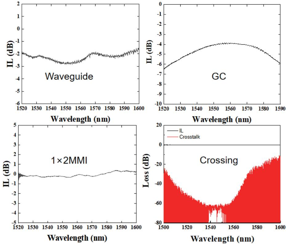
Fig. 3. (Color online) Performance results for passive PZT devices in the C-band.
