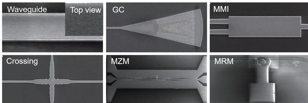
Fig. 2. (Color online) High-resolution SEM images of PZT devices.
