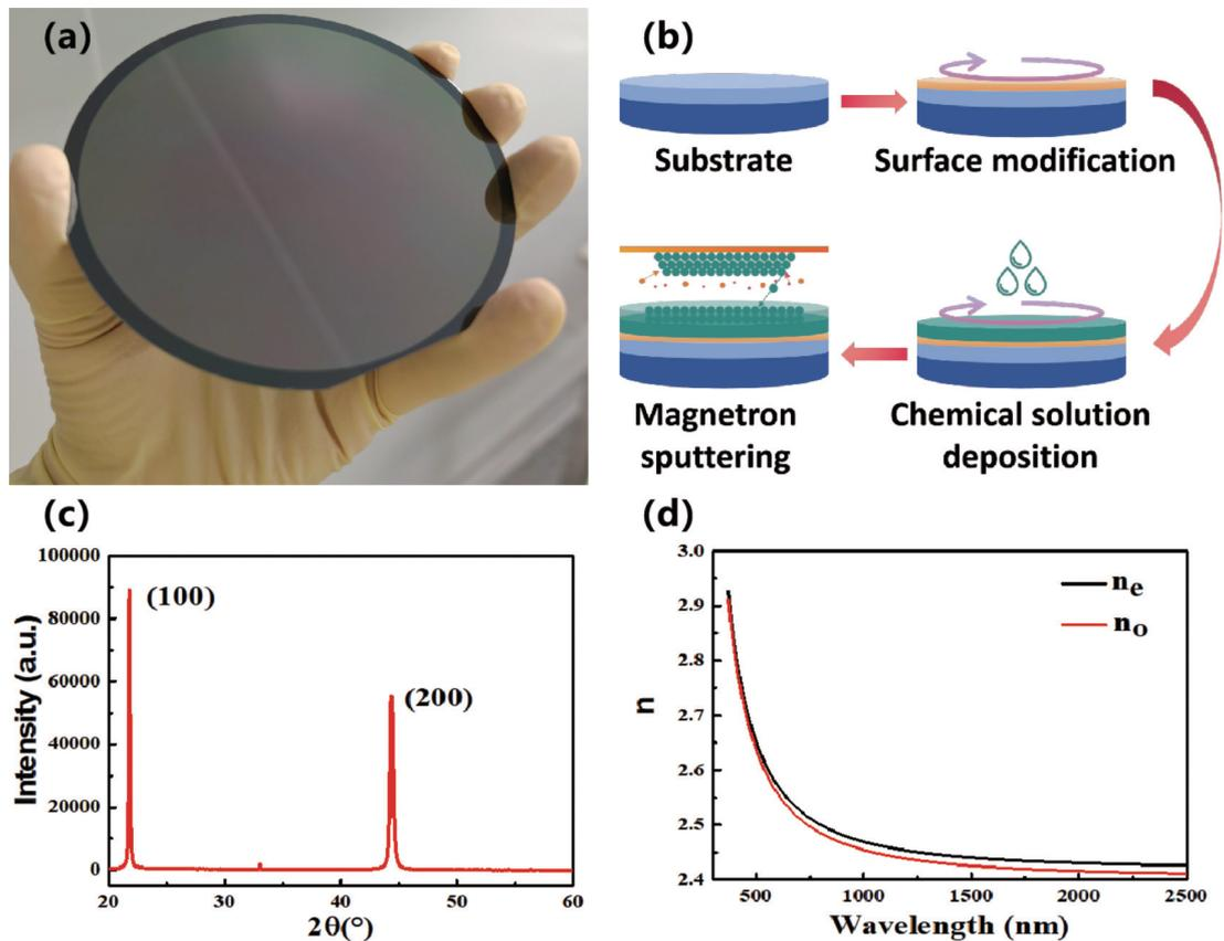
Fig. 1. (Color online) (a) Fabricated 4-inch PZT wafer. Fabrication process (b), XRD results (c) and ellipsometric measurements (d) of the PZT films.
