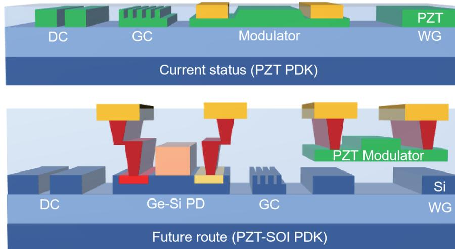
Fig. 4. (Color online) Development from PZT optical platform to PZT-SOI optical platform.
